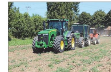
Figure 3. Traction test layout. The rear tires of the first tractor undergo testing. The vehicle in the middle is the DV. It is a modified tractor able to develop longitudinal force at the test tractor drawbar and be set up with a force transducer on the front and a fifth wheel on the rear for measuring forward speed. Some tests required an auxiliary tractor to increase the braking force (the red tractor in the picture).
