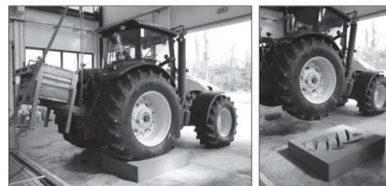
Figure 1. The footprint test layout.
